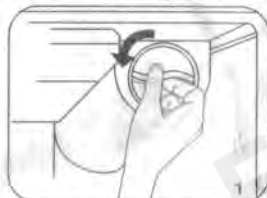
1) Remove the old cartridge by turning the filter cartridge handle counter-clockwise.
