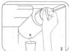
3) Pull out the cartridge from the filter housing.
