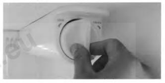
Roll the filter cartridge with pushing for correct insert position of the cartridge.
